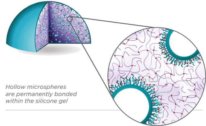
*Hollow microspheres are permanently bonded within the silicone gel*
